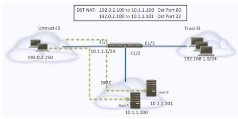
A network administrator is using DNAT to map two servers to one public IP address. Traffic will be directed to a specific server based on the application, where Host A (10.1.1.100) receives HTTP traffic and Host B (10.1.1.101) receives SSH traffic. Which two sets of Security policy rules will accomplish this configuration? (Choose two.)
