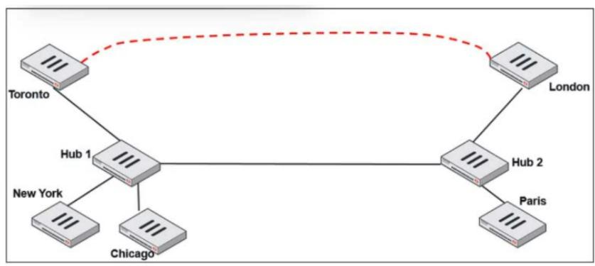
Two hub-and-spoke groups are connected through a site-to-site IPsec VPN between Hub 1 and Hub 2.
