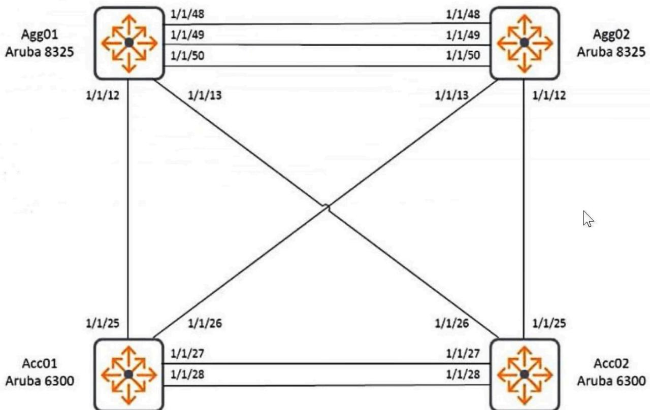
An engineer has attempted to configure two pairs of switches in the referenced configuration. It is required to implement Multi-Chassis Link Aggregation for each pair of switches.
