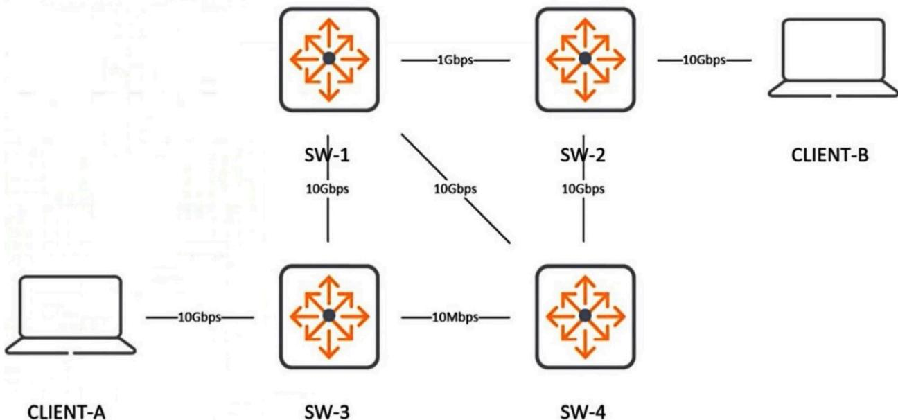
With the ports set up as routed ports, and default parameters for OSPF, what is the OSPF cost for the connection between SW-3 and SW-4?
