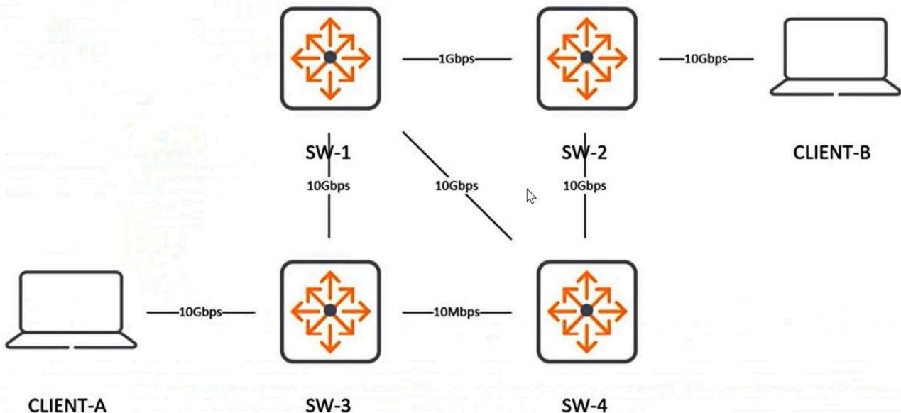
All ports are routed, and ECMP is enabled, with other default parameters for OSPF. What will be the result of traffic sent from CLIENT-A to CLIENT-B?
