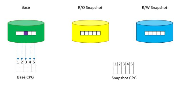
You create two snapshots of a thin provisioned base volume in an HPE Primera. One snapshot is read only and the other is read-write. A write occurs at the location shown in in the diagram.
