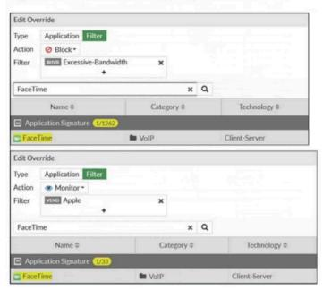
The exhibits show the application sensor configuration and the Excessive-Bandwidth and Apple filter details.
