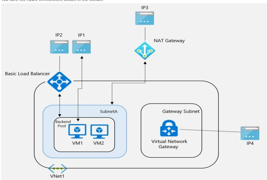
VM1 is a virtual machine that has an instance-level public IP address (ILPIP).
