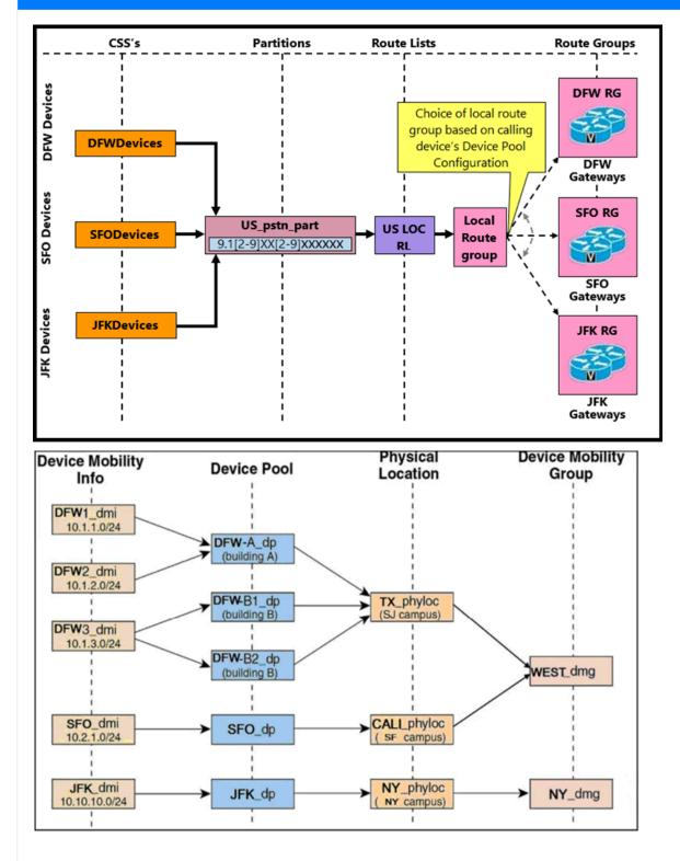
Refer to the exhibit. A user takes a phone from San Francisco to New York for a short reassignment. The phone was set up to use the San Francisco device pool, and device mobility is enabled on the Cisco UCM. The user makes a call that matches a route pattern in a route list that contains the Standard Local Route Group.
