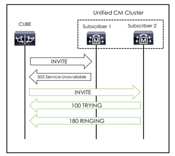
Cisco Unified Border Element is attempting to establish a call with Subscriber 1, but the call fails. Cisco Unified Border Element then retries the same call with
