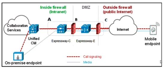
Refer to the exhibit. When making a call to a MRA client, what are the combinations of protocol on each of the different sections A-B-C?
