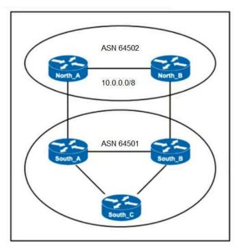
Refer to the exhibit. ASN 64501 currently reaches the networks under the 10.0.0.0/8 prefix via the North\_B router, which is a slow backup link. The administrator of ASN 64502 wants traffic from ASN 64501 to 10.0.0.0/8 to travel via the primary link, North\_A. Which change to the network configuration accomplishes this task?
