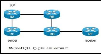
Refer to the exhibit. If router RA is configured as shown, which IPv4 multicast address space does it use?
