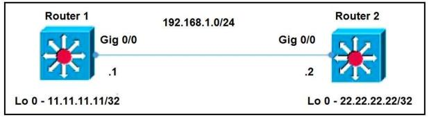
Refer to the exhibit. Router 1 and router 2 are running OSPF Area 0. The router logs on both routers show that the LDP link has flapped. Which configuration must the engineer apply to the two routers to implement session protection on the link?
