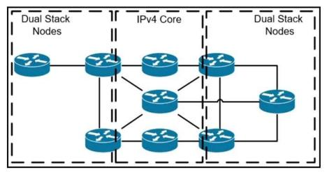
Refer to the exhibit. A network operator has two IPv4 and IPv6 dual-stacked networks on each side of the IPv4 core network. The operator must be able to provide connectivity between them while using specific assigned IPv6 space provided from the company IP administrator team. Which technology should the network operator use to accomplish this goal?
