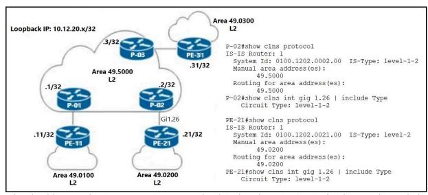
Refer to the exhibit. A network engineer notices PE-21 convergence degradation due to the growing LSDB size of Level 2 areas in the network. The engineer decides to migrate router PE-21 from an inter-area design to an intra-area implementation. Inter-area routing must be accomplished via an ATT-bit set by the
