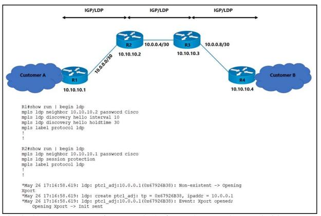
Refer to the exhibit. The operations team is implementing an LDP-based configuration in the service provider core network with these requirements:
