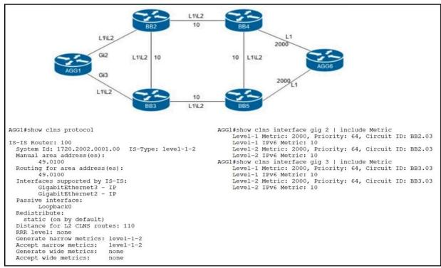
Refer to the exhibit. An engineer is configuring IS-IS on ISP network. Which IS-IS configuration must an engineer implement on router AGG1 so that it establishes connectivity to router AGG6 via the BB3 core router?
