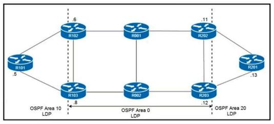
Refer to the exhibit. R101 is peering with R102 and R103, and R201 is peering with R202 and R203 using iBGP Labeled Unicast address families. The OSPF area 0 border routers are in a full iBGP Labeled Unicast mesh, and VPNv4 routes are exchanged directly between PE routers R101 and R201 through iBGP.
