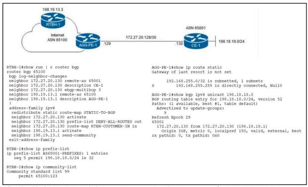
Refer to the exhibit. ISP ASN 65100 provides Internet services to router CE-1 and receives customer prefix 198.18.18.0/24 via eBGP. An administrator for the ISP is now provisioning RTBH services to provide on-demand data-plane security for the customer's IP space. Which routemap configuration must the administrator apply to router RTBH-1 to complete the implementation of RTBH services to CE-1?
