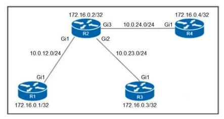
Refer to the exhibit. Which configuration must be applied to each of the four routers on the network to reduce LDP LIB size and advertise label bindings for the /32 loopback IP space only?
