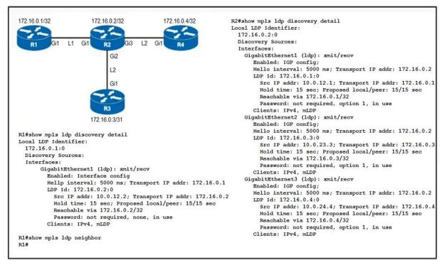
Refer to the exhibit. An engineer began to configure LDP between R1 and R2, but R1 and R2 cannot yet establish an LDP TCP connection. Which additional task must be completed to finish the implementation?
