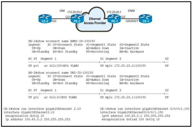
Refer to the exhibit. An Ethernet access provider is configuring routers PE-1 and PE-2 to provide E-Access EVPL service between UNI and ENNI. ENNI service multiplexing is based on 802.1ad tag 150, and service-multiplexed UNI is based on 802.1q tag 10. Which EFP configurations must the provider implement on PE-1 and PE-2 to establish end-to-end connectivity between CE-1 and CE-2?
