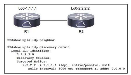
Refer to the exhibit. When implementing an LDP protocol, an engineer experienced an issue between two directly connected routers and noticed that no LDP neighbor exists for 1.1.1.1.
