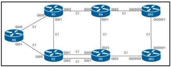
Refer to the exhibit. An engineer configured R6 as the headend LSR of an RSVP-TE LSP to router XR2, with the dynamic path signaled as R6-R2-R5-XR2, and set the OSPF cost of all links to 1. MPLS autotunnel backup is enabled on all routers to protect the LSP. Which two NNHOP backup tunnels should the engineer use to complete the implementation? (Choose two.)
