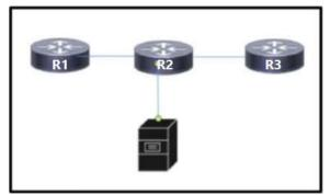
Refer to the exhibit. Users on a network connected to router R3 report slow speeds when they connect to the server connected to R2. After analyzing traffic on the network, a network engineer identified congestion on the link between R2 and R3 as the cause. Which QoS service must the engineer implement to drop traffic on the link when it exceeds a configured threshold?
