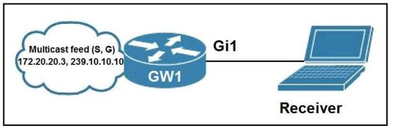
Refer to the exhibit. A network administrator is implementing IGMP to enable multicast feed transmission to the receiver. Which configuration must the administrator deploy on GW1 to permit IGMP joins only to the assigned (S, G) feed?
