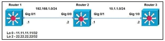
Refer to the exhibit. Router 1 and router 2 are running IBGP, and router 2 and router 3 are running OSPF Area 0. Router 1 is advertising loopback interfaces Lo 0 and Lo 2, and router 2 is redistributing BGP into OSPF Area 0. Which configuration must an administrator apply so that router 2 uses a route map to redistribute only the internal route from Lo 2?
