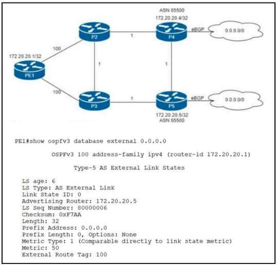
Refer to the exhibit. Routers P4 and P5 receive the 0.0.0.0/0 route from the ISP via eBGP peering. P4 is the primary Internet gateway router, and P5 is its backup.
