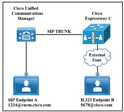
Refer to the exhibit. In an environment SIP devices are registered to CUCM and H.323 devices to VCS. What would be required to enable these calls to setup correctly?
