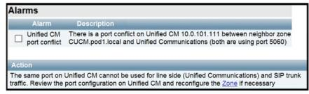
Refer to the exhibit. Mobile and remote access is being added to an existing B2B deployment and is failing. When the administrator looks at the alarms on the
