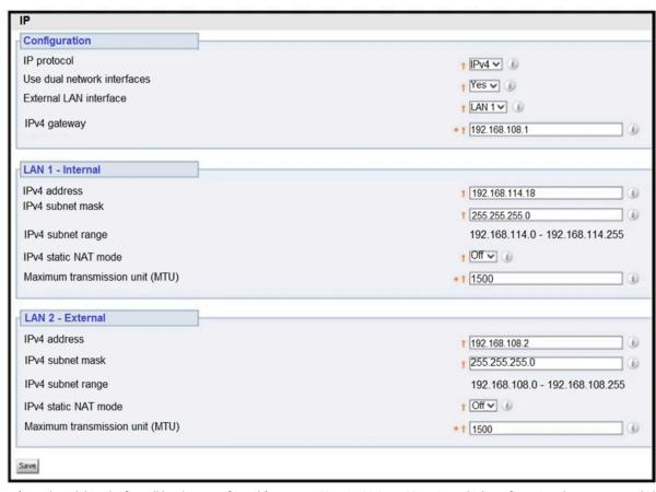
Refer to the exhibit. The firewall has been configured from NAT 192.168.108.2 to 100.64.0.1. Which configuration changes are needed for an Expressway-E with dual network interfaces?
