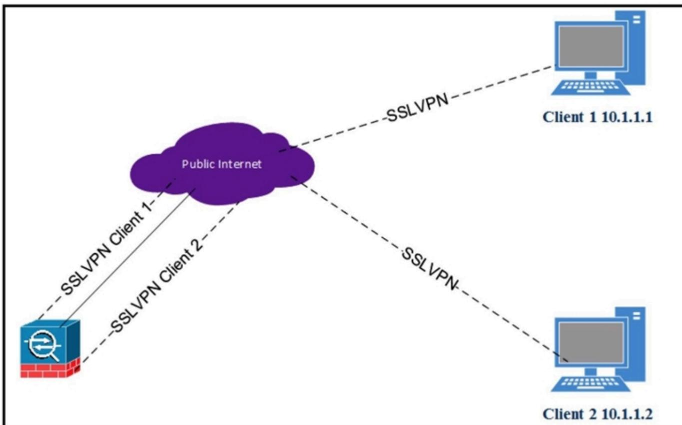
Refer to the exhibit. Client 1 cannot communicate with client 2. Both clients are using Cisco AnyConnect and have established a successful SSL VPN connection to the hub ASA. Which command on the ASA is missing?
