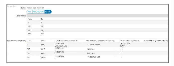
Refer to the exhibit. A Cisco ACI fabric is using out-of-band management connectivity. The APIC must access a routable host with an IP address of 192.168.11.2. Which action accomplishes this goal?
