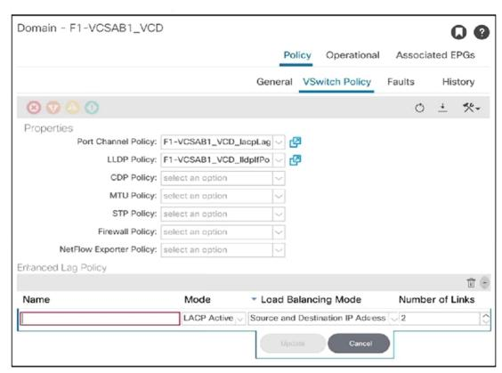
Refer to the exhibit. An engineer configures the Cisco ACI fabric for VMM integration with ESXi servers that are to be connected to the ACI leaves. The server team requires the network switches to initiate the LACP negotiation as opposed to the servers. The LAG group consists of two 10 Gigabit Ethernet links. The server learn also wants to evenly distribute traffic across all available links. Which two enhanced LAG policies meet these requirements? (Choose two.)
