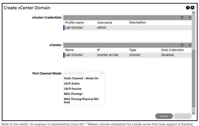
Refer to the exhibit. An engineer is implementing Cisco ACI "VMware vCenter integration for a blade server that lacks support of bonding. Which port channel mode results in "route based on originating virtual port" on the VMware VDS?
