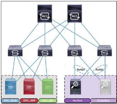
Refer to the exhibit. A Cisco ACI fabric is newly deployed, and the security team requires more visibility of all inter EPG traffic flows. All traffic in a VRF must be forwarded to an existing firewall pair. During failover, the standby firewall must continue to use the same IP and MAC as the primary firewall. Drag and drop the steps from the left into the implementation order on the right to configure the service graph that meets the requirements. (Not all steps are used.)
