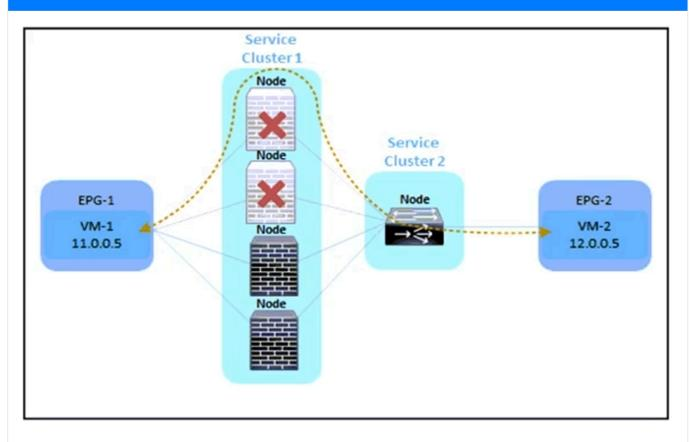
Refer to the exhibit. An engineer must divert the traffic between VM-1 and VM-2 by using a Multi-Node service graph. The solution should prevent an insufficient number of available Layer 4 to Layer 7 devices in the first cluster. Which configuration set accomplishes this goal?
