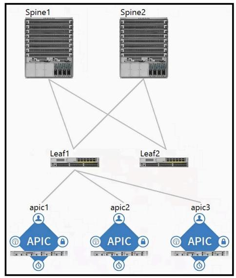
Refer to the exhibit. Which two components should be configured as route reflectors in the ACI fabric? (Choose two.)
