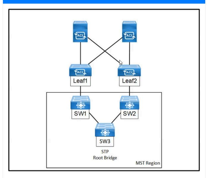
Refer to the exhibit. An engineer is deploying a Cisco ACI environment but experiences a STP loop between SW1 and SW2. Which configuration step is needed to break the STP loop?
