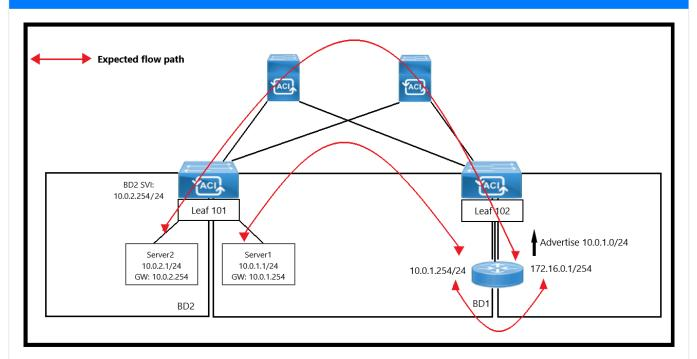
Refer to the exhibit. An engineer wants to initiate an ICMP ping from Server1 to Server2. The requirement is for the BD1 to enforce ICMP replies that follow the expected path. The packets must be prevented from taking the direct path from Leaf1 to Server1. Which action must be taken on BD1 to meet these requirements?
