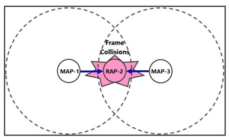
Refer to the exhibit. During a post Mesh deployment survey, an engineer notices that frame collisions occur when MAP-1 and MAP-3 talk to RAP-2. Which type of issue does the engineer need to address in the design?
