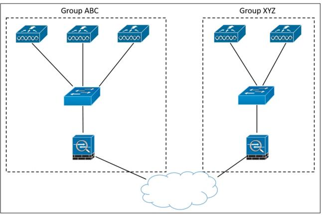
Refer to the exhibit. An enterprise has offices spread around the globe. The APs are connected to different controllers installed in separate datacenters. The IT team wants to allow clients to roam from controllers in group ABC to controllers in group XYZ. Which feature must be incorporated in the design to accomplish this task?
