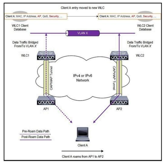
Refer to the exhibit. A client roams between two APs that are registered to two different controllers, where each controller has an interface in the client subnet.
