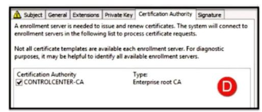
An administrator configures a CA certificate for the Connection Server. However, they are still encountering certificate warnings when trying to connect to the Connection Server. The exhibit displays the properties of the CA-Signed certificate.
